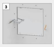
Adjust the frame (check angularity), fasten it and mark the drill holes, Drill distance ≤200 mm. Drill distance in case of access panel Alumatic "air-tight and dust-tight": ≤ 100mm.
