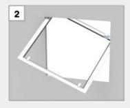
Hang out the detachable flap lid, insert diagonally the panel frame through the opening and place it
