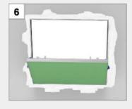
Then perform functional test (insert, close, open). Fit the flap lid, fix the arresting device and close the flap lid.
