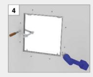
Drill with a drilling machine of 3mm through the gypsum and
