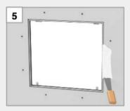
Fill the mounting frame and the flap lid separately using a joint filler. Clean the metallic interior and side surfaces of the mounting frame and the door leaf after further coating of putty and paint residues!
