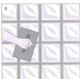
8. Apply the finishing, fill the joints well; use soft brushes and plastering trowels. Make a perimeter cordon, or part of the outside joint, using elastic sealant to prevent cracking along the expansion/settling joints. If the walls are to be exposed to water, use a transparent protective paint along the joints to enhance their water-proof features.
